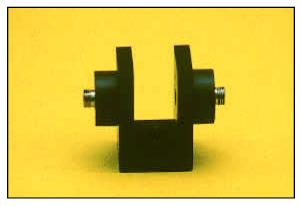
Fiber optic U-bracket assemblies are designed to transmit light from an optical fiber, across an air gap, and back into a second fiber with low losses. The U-bracket is prealigned at the factory for minimum insertion losses, making it very easy to use. A variety of bulk optical devices, including polarizers, isolators, filters, and waveplates, can be simply inserted into the U-bracket, allowing the user to quickly and easily test or prototype systems incorporating fiber and bulk optics.
